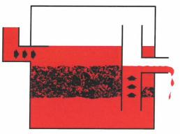
Liquefies solids—for faster penetration and improved liquid flow.
